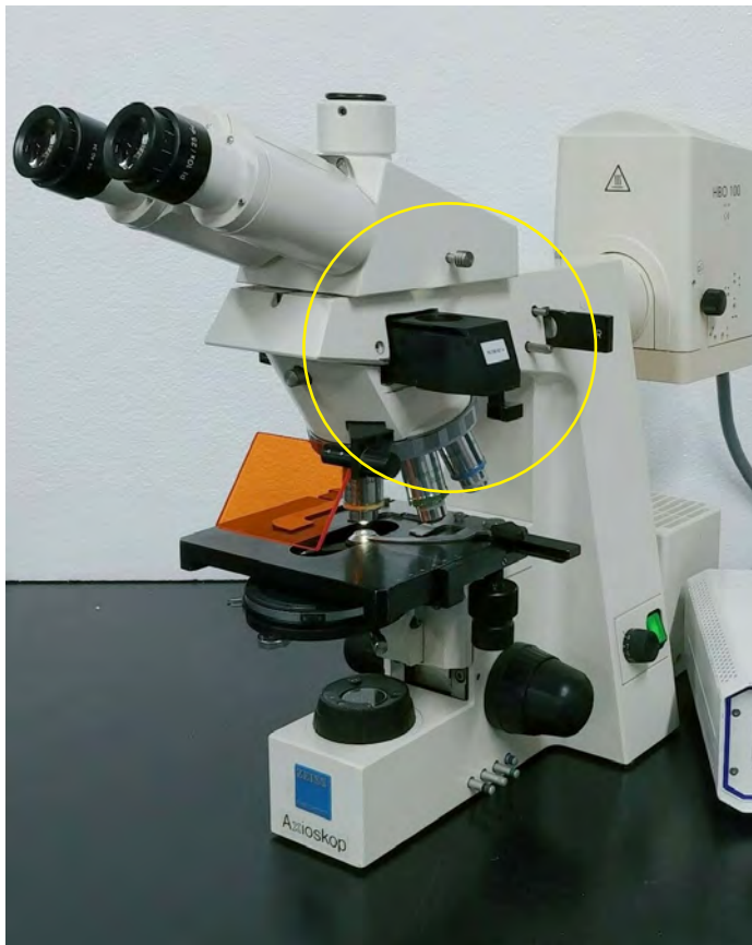
Zeiss Axioskop Fluorescent filter slider consists of Emission filter (5), Excitation filter (4), and Dichroic beamsplitter (2). The filter block is identical to slider in Axiovert 100.
